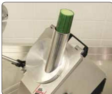
Use the angle cut feeder to cut vegetables for professional wok dishes and decorative slices of cucumber etc.
