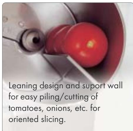
Leaning design and support wall for easy piling/cutting of tomatoes, onions, etc. for oriented slicing.
