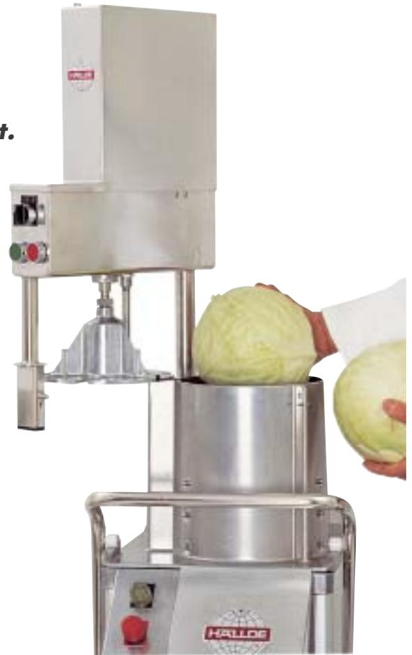
**Feed hopper with its own type A feed cylinder for continuous feeding/cutting of potatoes, onions, dry bread, nuts, almonds, mushrooms, etc.**
